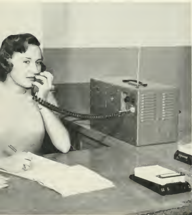
Dispatcher (left) at Standard Pressed Steel plant in Jenkintown, Pa., is able to reach the operator of any lift truck (below) in factory or yards, over the RCA two-way radio system.
